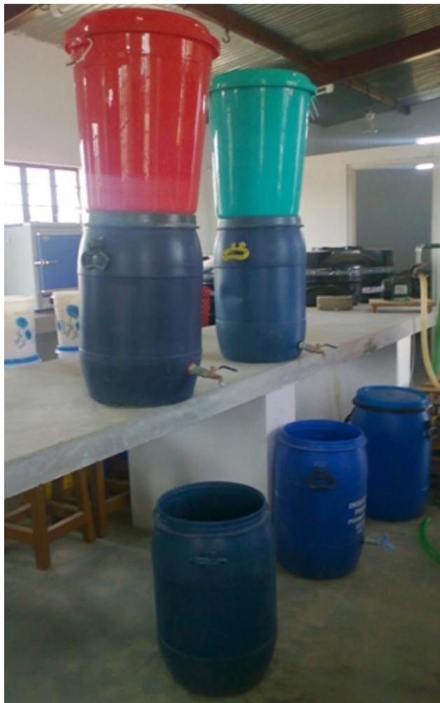
**Figura 3.** Photo of the fabricated filter with four ceramic candles with Activated Alumina
