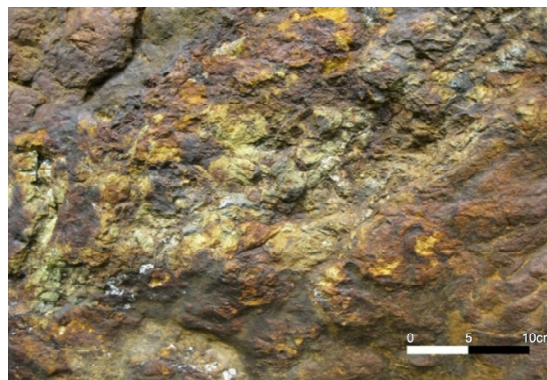
Fig. 3. Fragment of massive quartz-pyrrhotite-chalcocopyrite ore, Gelia vein.
