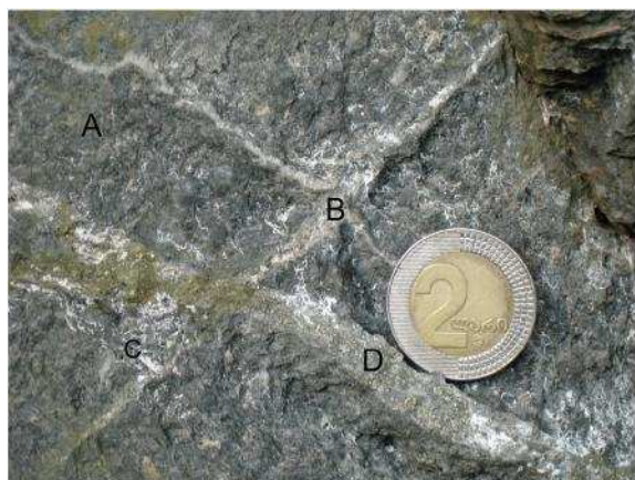
Figure 3. Silicified and ore mineralized Lower Jurassic shale, r.Stori canyon. A. silicified, sericitized and carbonatized shale; B. quartz vein, C. carbonate veins, D. quartz-pyritepyrrhotite vein.
