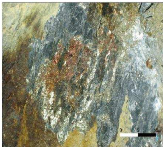
Figure 4. Ore-bearing quartz-pyrrhotite-chalcopyrite veinlets in selvage of vein " Inglisuri ".
