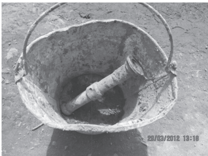
Picture 8. ^{137}\text{Cs} radioactive source found in scrap metal
