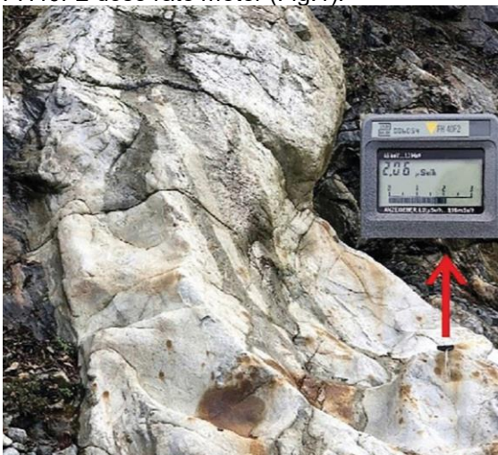
Figure 1. One of the Shkhara plagiogranite vein with FAG-FH40F2 dosimeter showing the dose 2.06 \mu\text{Sv}/\text{h} .
